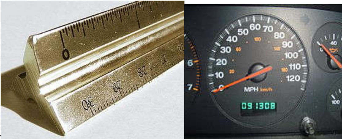
A triangular architect's scale, made of brass
